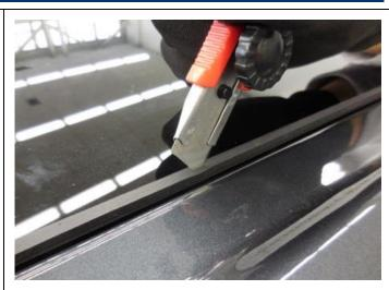
5. Using a sealant cutter, cut the sealant (D)
