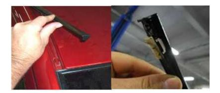
Shown above are examples of clear, close-up pictures to better show the detail of the issue (These example pictures show the ditch molding area on the vehicle and the actual area on the molding part that comes loose and/or is lifted).
