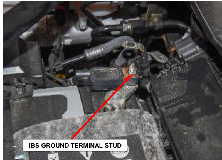
Figure 2 – IBS Ground Terminal Stud
