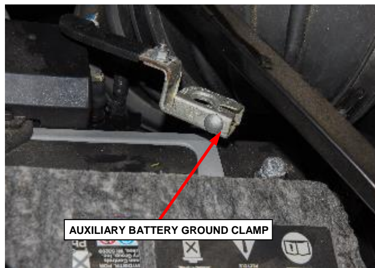
Figure 3 – Auxiliary Battery Ground Clamp
