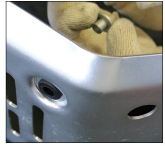
Apply "Loctite 243" medium strength threadlocker to the 4 screws M8x25 (code AP8152287) fixing the sump guard to the support bracket and then tighten to a torque of 15 Nm or (11 lb. ft.).
