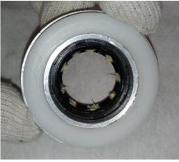
Fully insert the seal/cover on the spacer sleeve in the final drive, taking care to use the plastic tie included in the kit. This tie will allow air to escape, which will allow the complete insertion of the cover in its seat. Remove the plastic tie.
