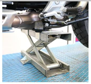
Remove the rear wheel after removing the caliper support, without disconnecting the brake hose.
