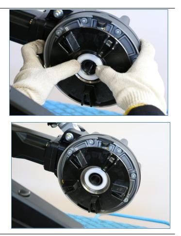
Refit the rear wheel and the brake caliper support and torque to the specified torque values.
