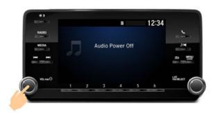
27. Press and hold the VOL/Power AUDIO knob to bypass the anti-theft screen.
