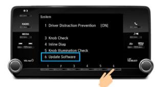
17. When the **Update Software** screen appears, press the SELECT knob to start the update mode. The audio unit automatically reboots, and the **Update Software SYS** screen appears.
