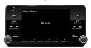
22. When the **Update Software** screen appears again in approximately **5 seconds**, press the SELECT knob to start the update mode. The audio unit automatically reboots, and the **Update Software SYS** screen appears.
