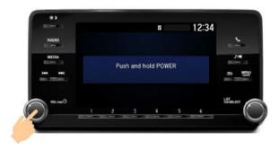
28. When the FM station is displayed, press the VOL/Power AUDIO knob to turn the audio unit to OFF.
