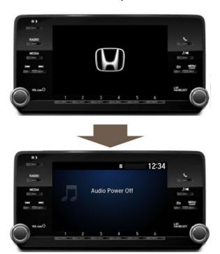
26. Press the VOL/Power AUDIO knob to turn the audio unit to ON.
