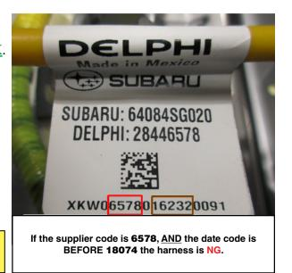
\*\*NOTE: In the VERY RARE case where the harness is OK but the AIRBAG warning light is on with an ODS -related DTC in memory, submit a recall claim for inspection only. Continue diagnosing the DTC following the modified Service Manual procedure provided on pg. 8 for reference as there may be another cause for this DTC. Refer to the Vehicle Coverage Inquiry to identify available coverage.
