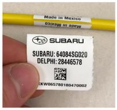
Step12- Remove the adhesive backing and apply the cut off section of the original label to the new replacement harness as shown in the photo sequence below.
