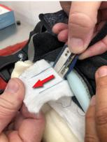
Step8- IMPORTANT: Before connecting the new harness, inspect the tail and sensor mat connectors to confirm they are tight on the 2 metal bands of the mat. Inspect closely for any breaks, cracks or other damage to the visible components of the sensor mat. If any damage is identified, the complete seat cushion assembly must be replaced as the sensor mat is not a serviceable component.
