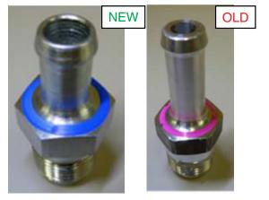
NOTE: P.n. SOA635322 (ThreeBond 1217H) is to be used for the PCV valve thread sealer.
