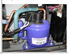
Q: Thermal Limit Switch on Compressor:
