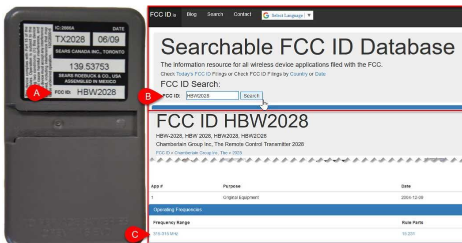
Figure 1. Checking the operating frequency.
