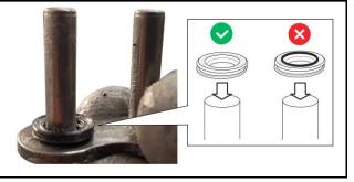
**6.** Insert the fork of the new master link from the rear part of the chain, avoiding any contact with the pins so as not to remove any lubricant
