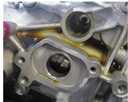
Fault type 2: Cylinder head cover leaking
