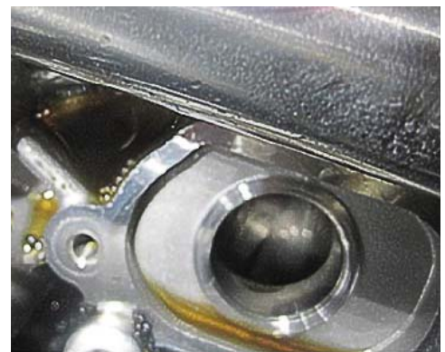
Fault type 1: Valve lift adjustment solenoid hydraulic leaking
