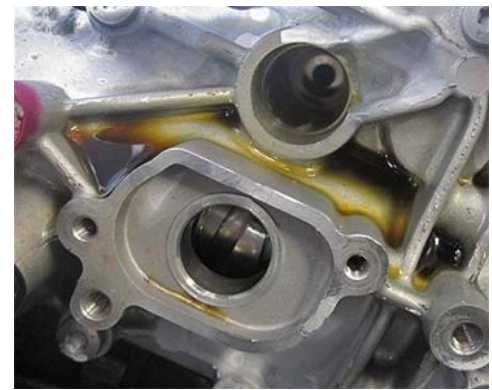
Fault type 2: Cylinder head cover leaking
