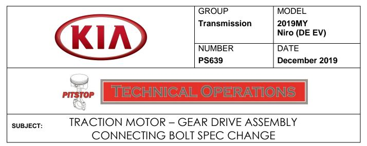
This bulletin provides information on the installation of the <u>four</u> (4) longer (75mm) connecting bolts between the Traction Motor and Gear Drive Assembly on some 2019MY Niro (DE EV) produced before May 13, 2019, which is noted in the EPC when ordering a traction motor assembly for replacement.
