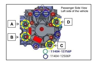
Torque specifications for <u>all</u> traction motor retaining bolts: 58.6 – 71.6 lb.ft (79.4 – 97.1 Nm., 8.1 – 9.9 kgf.m)
