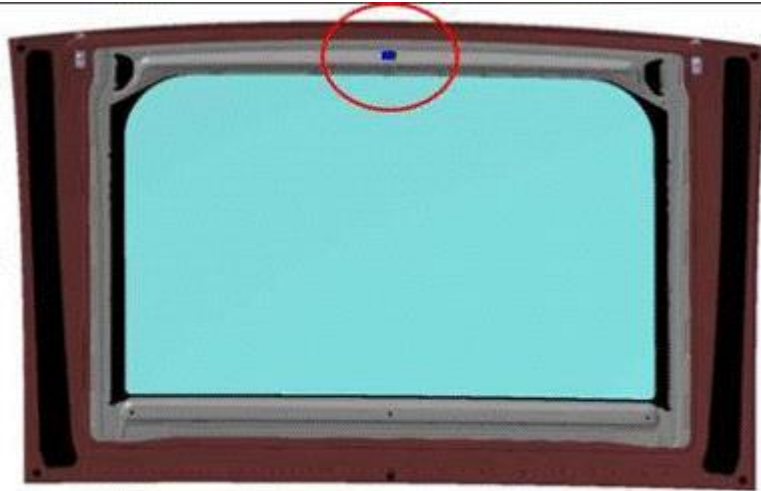
Figure 15. Area of sunroof glass panel structure to be prepared.
