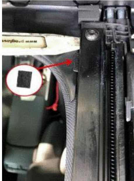
Figure 13. Isolation of guide rail and frame by the installation of a section of felt strip material.
