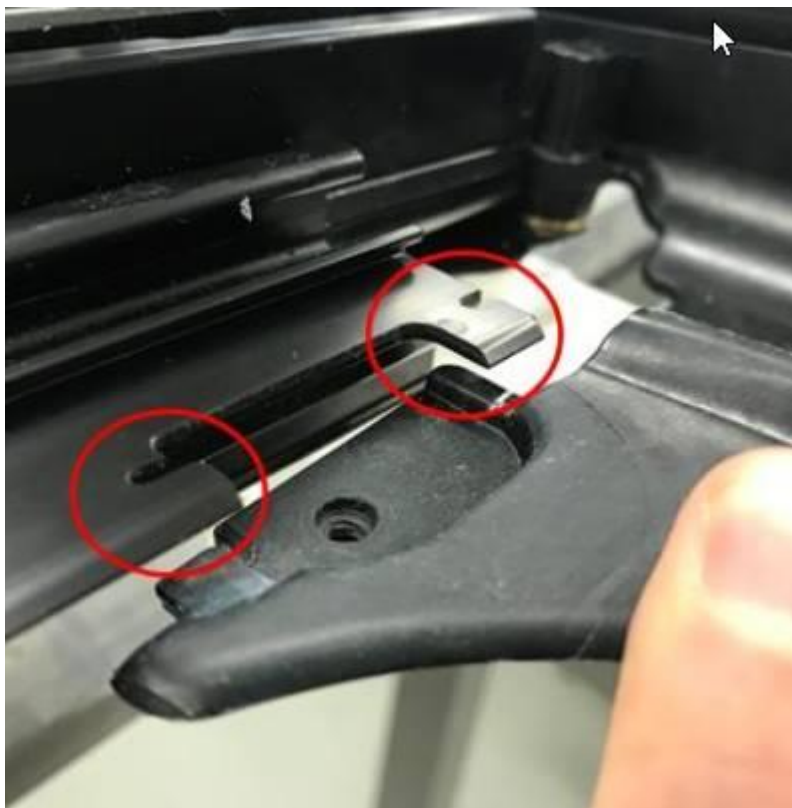
Figure 7. Areas to clean using cleaning solution D 009 401 04.
