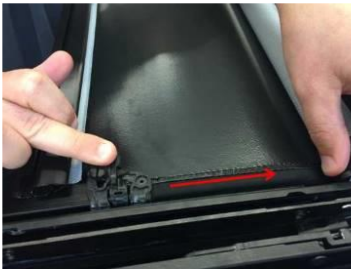
Figure 4. Push the material back to expose the bolts.
