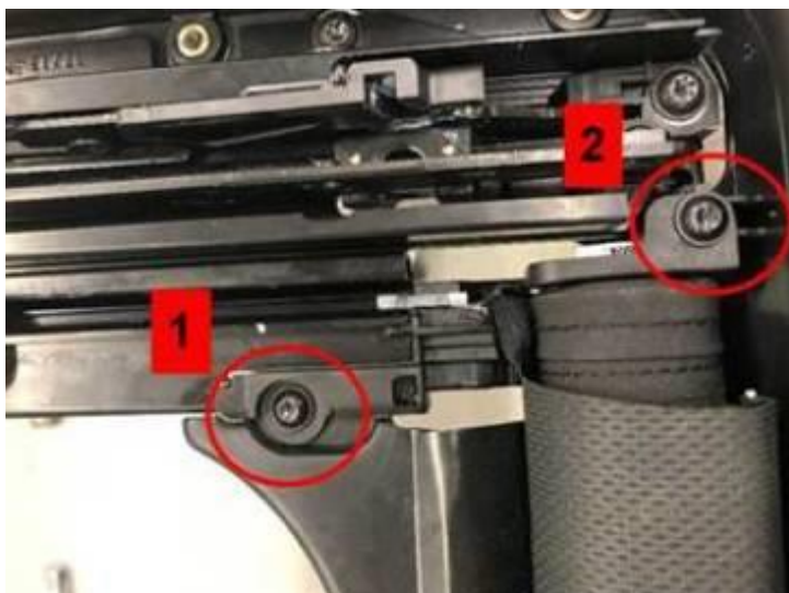
Figure 5. Remove the bolts.
