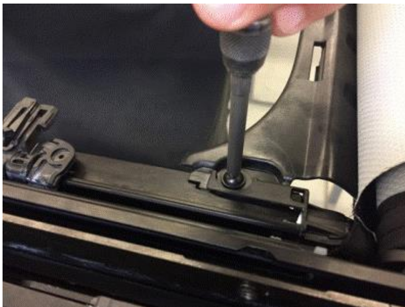
Figure 11. Torque screws to 3Nm.
