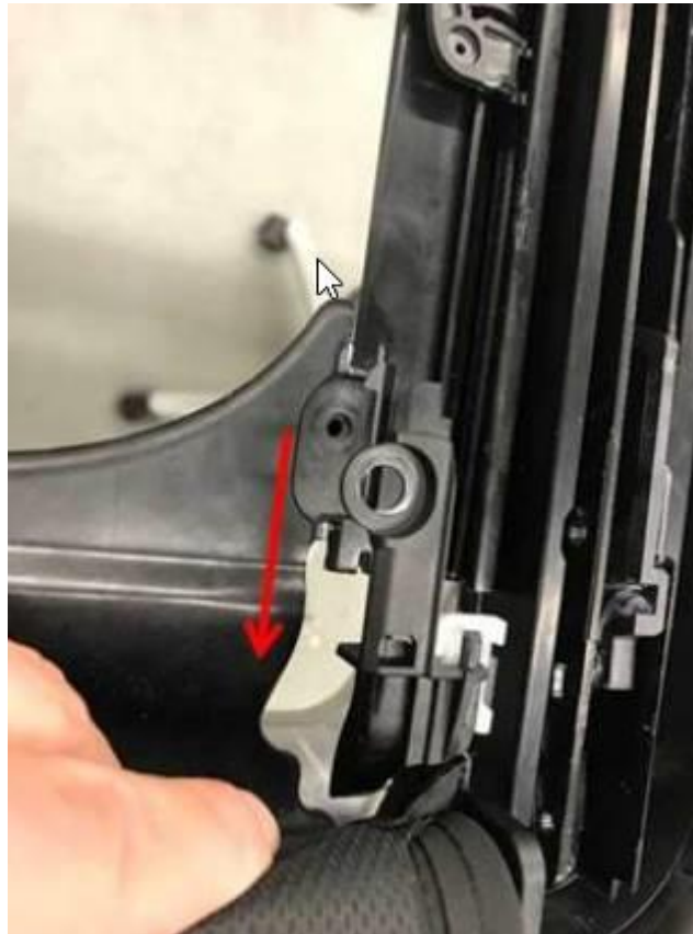
Figure 6. Slide roller shade backward.
