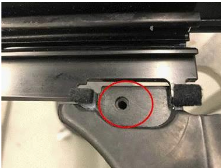
Figure 10. Apply thread locker in this area.
