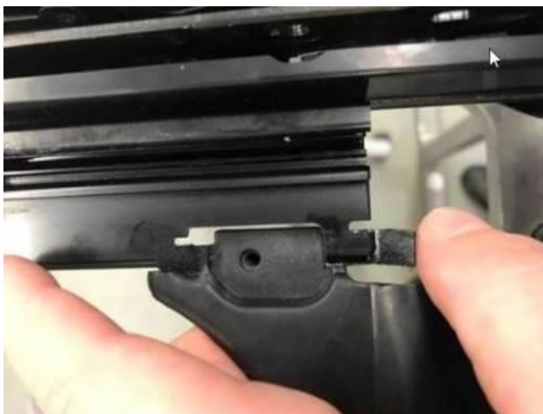
Figure 7. Areas to clean using cleaning solution D 009 401 04.
