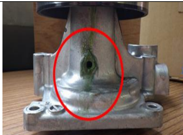
Dried coolant steam shows as green-color deposit at bleed hole
