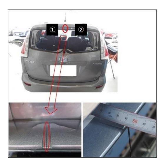
The crack occurs beneath the high mount stop light, with cracking towards the front direction. This might be caused by insufficient adhesive application when the rear glass was removed.
