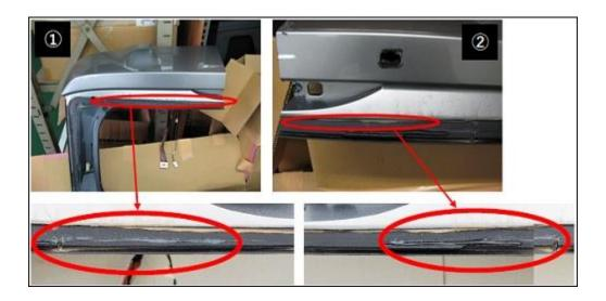
**NOTE:** The glass needs to be pressed perpendicular to the frame during installation. Appropriate glass installation and adhesive application in between glass and outer layer of lift gate panel are essential to prevent the lift gate crack after rear glass replacement.
