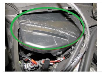
**YES** - This is a filter box lid with the integrated water guiding channels.
