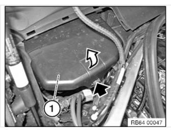
Unlock the retaining tab (black arrow) and lift the filter box lid (1) up.
