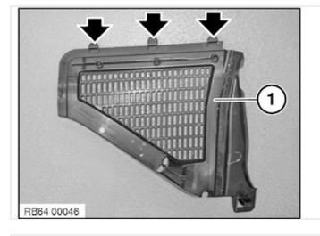
Note: The tabs (arrows) on the cover (1) must engage correctly under the cowl panel.
