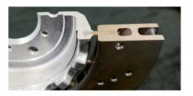
M Compound brakes have a grey-cast friction ring in a floating arrangement that is connected by pins to the aluminum rotor hat. The pin assembly means that as the temperature increases, it is able to expand freely in a radial direction and subsequently cool down again without any residual deformation.
