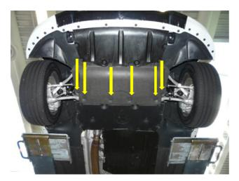
• Release the six fastening screws (yellow arrows) to expose the front area of the axle support
