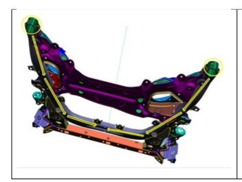
**Note-** The cavity wax will need to reach the front area of the axle support as indicated by the yellow arrows (viewed looking up from beneath vehicle).
