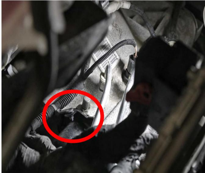
**Figure 3 – Fir Tree Retainer**
