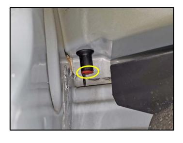
Remove flaps from left front and right front sunroof drains.
