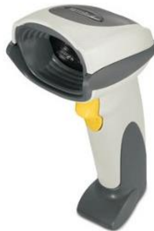
Figure 1. 2D scanner VAS 6161/1.
