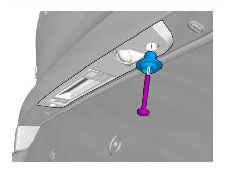
Install component/components from the repair kit.
