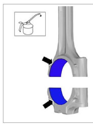
Warning! Make sure that the component is positioned correctly.
