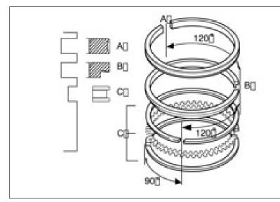
Caution! Make sure that the piston rings can be easily rotated by hand in the piston ring grooves.
