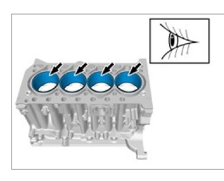
Note! If there are scratches in the cylinder bore, which are confirmed by feeling with the nail, the engine must be replaced
