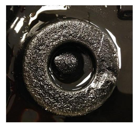
The following picture shows particle buildup that may appear as fuzz, strands or chips. Using gloves, rub a small amount of the magnetic debris between your fingers or onto a hard surface. If the debris breaks down and feels almost smooth, please continue diagnosis. If there are actual chips in the debris, the transmission should be replaced.
