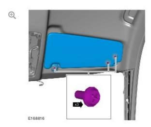
Remove the 3 bolts and remove the sun visor.
