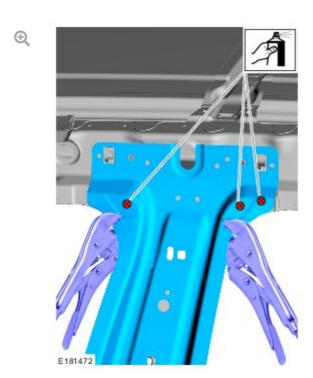
Use a suitable corrosion protection to cover the repaired area.
