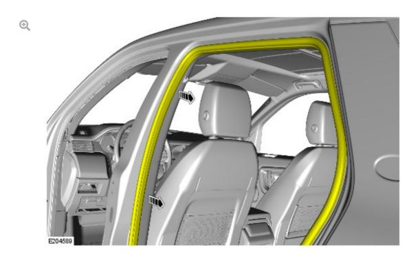
Release and position to one side the rear door aperture seal from the door aperture.
