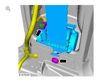
Install the seatbelt retractor.
