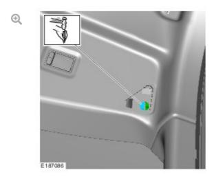
Insert a parallel pin punch with a minimum diameter of 16 mm, through the sun visor bracket aperture. Using a hammer, strike the punch in an upward motion several times. This allows the panels to be distorted away from the sun visor bracket aperture. This can eliminate noises which originate from this area.
