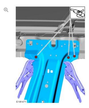
Grind away any excess material where the vehicle has been MIG welded.
