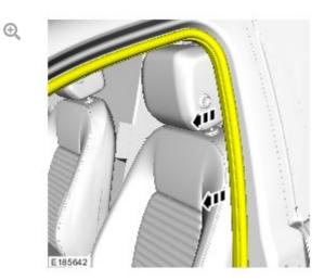
Release and position to one side the front door aperture seal from the door aperture.
