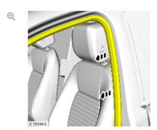
Release and position to one side the front door aperture seal from the door aperture.
