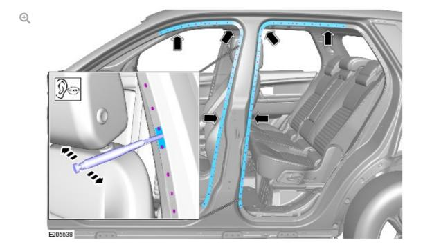
Move the panels around the door apertures, first inwards and then outwards as shown until no click can be heard. Complete this step to the areas highlighted. This can eliminate noises which originate from this area.
