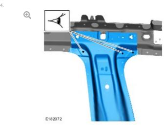
Identify the 3 spot welds to be drilled.
