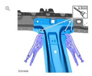
Drill the 3 spot welds to the correct depth of 2.5 mm.
