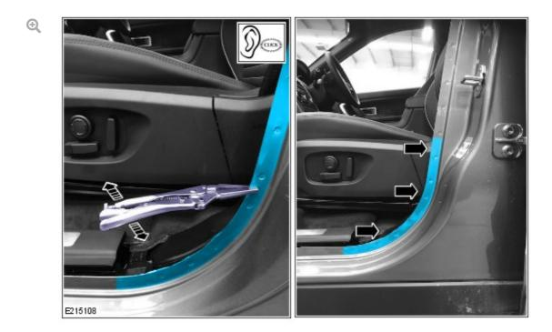
Move the panels around the door apertures, first inwards and then outwards as shown until no click can be heard. Complete this step to the areas highlighted. This can eliminate noises which originate from this area.
