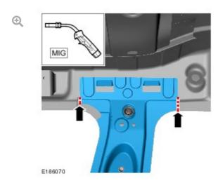
MIG seam weld the B-pillar in the area shown. This can eliminate noises which originate from this area.
