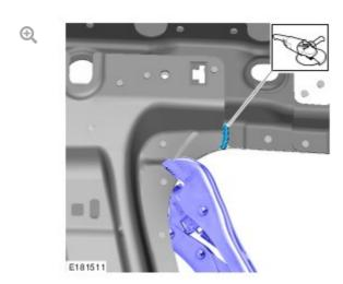
Grind away any excess material where the vehicle has been MIG welded.
