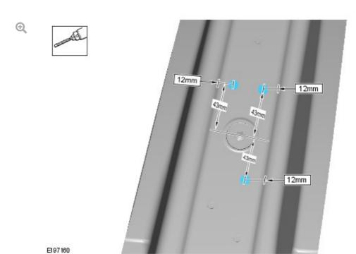
Drill three 6.5 mm diameter holes in the areas shown to a depth of 6 mm. This can eliminate noises which originate from this area.
