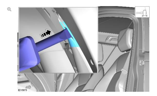
Using a suitable hammer, insert the suitable chisel between the inner B-pillar and the cant rail, to a maximum depth of 20 mm. This can eliminate noises which originate from this area.
