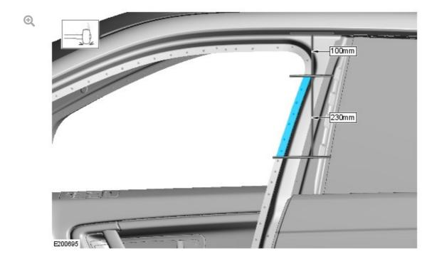
Using a suitable hammer, strike the panel inwards over the highlighted area shown. The panel should be struck with as much force as can safely be applied. Repeat along the highlighted area shown. This can eliminate noises which originate from this area.
