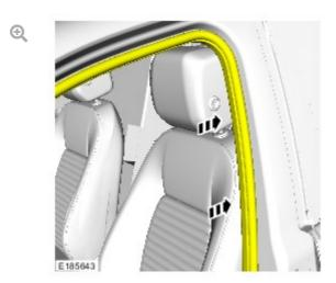
Install the front door aperture seal to the door aperture.
