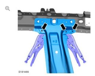
Make sure when installing the suitable tools to clamp the B-pillar, the spot welds that are to be drilled remain visible.
