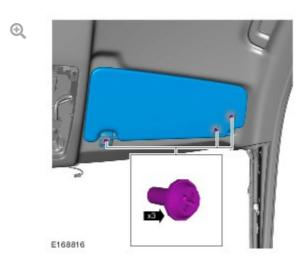
Install the sun visor and tighten the 3 bolts.
