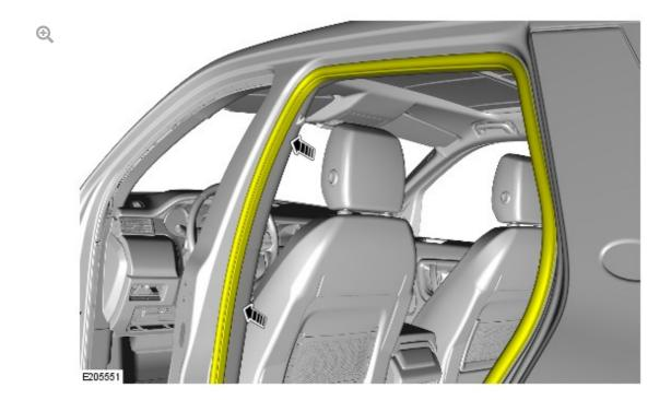
Install the rear door aperture seal to the door aperture.
