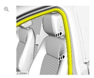
Install the front door aperture seal to the door aperture.
