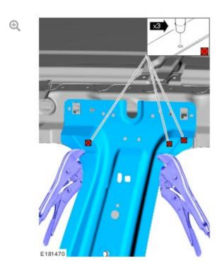
Metal Inert Gas (MIG) weld the 3 drilled holes.
