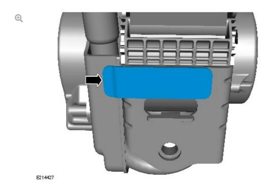
Install a 150 mm x 550 mm rectangular piece of 0.5 mm foam (from the Land Rover squeaks and rattles kit, or a similar 250g density, 30% wool 70% viscose felt), as shown in the illustration.
