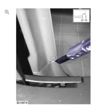
Using a suitable hammer, insert the suitable chisel between the B-pillar and rocker panel. Only 1 or 2 strikes with the suitable hammer should be required.
