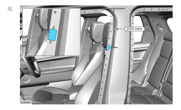
Place a single spot weld within the highlighted area shown. This can eliminate noises which originate from this area.
