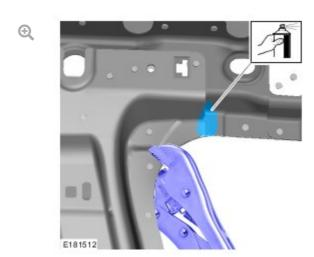
Use a suitable corrosion protection to cover the repaired area.
