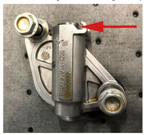
If the timing chain tensioner is found to be stuck or collapsed, replace the Timing Chain Tensioner, inspect the three timing chain guides for excessive wear or damage and replace as necessary.
