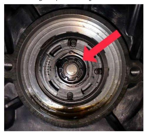
If the Snap Ring for either Camshaft Sprocket bolt is missing, out of position or damaged, replace both Camshaft Sprocket Bolts following the latest SI documents and perform the timing chain tensioner / guide inspections listed below.
