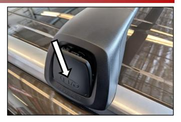
10. Push the top of the key cover to secure the cover to the cross bar end cap.
