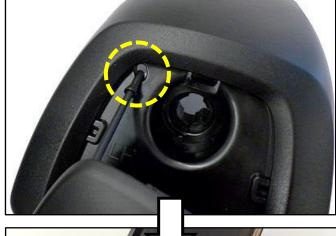
6b. On the reverse side of the cross bar end cap, pull the key cover plastic tether through the hole using a set of pliers to retain the key cover to the end cap.
