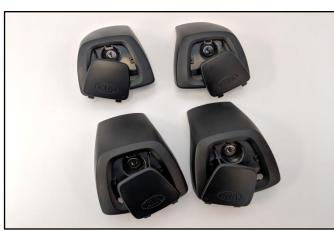
Reinstall the four (4) end caps onto the roof cross bars in the reverse order of removal. Ensure to lock all four (4) of the end caps with key.
