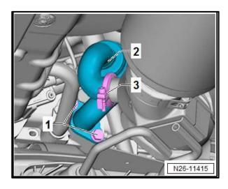
Inspect, and if necessary, replace EGR Filter <2>.
