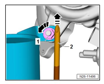
Apply screwdriver <2> on side of nut <1> and unscrew nut while simultaneously pressing up on nut.
