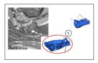
To correct this concern, the cold environment performance of the No.1 engine mount rubber has been increased by changing the rubber material.
