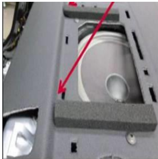
Figure 1. Foam strip installation for vehicles with Audi sound (PR code 9VD) .
