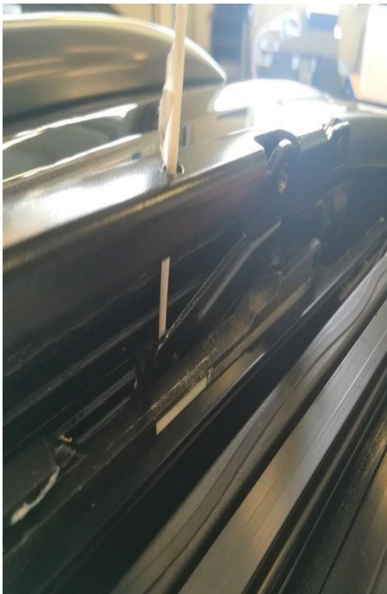
Figure 10. Close up view of the lubrication of the channel under the arm of the slide and tilt mechanism.
