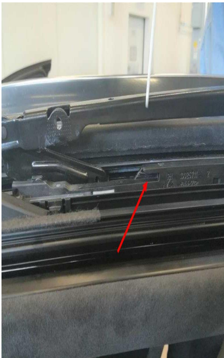
Figure 5. The groove in the slide and tilt mechanism.
