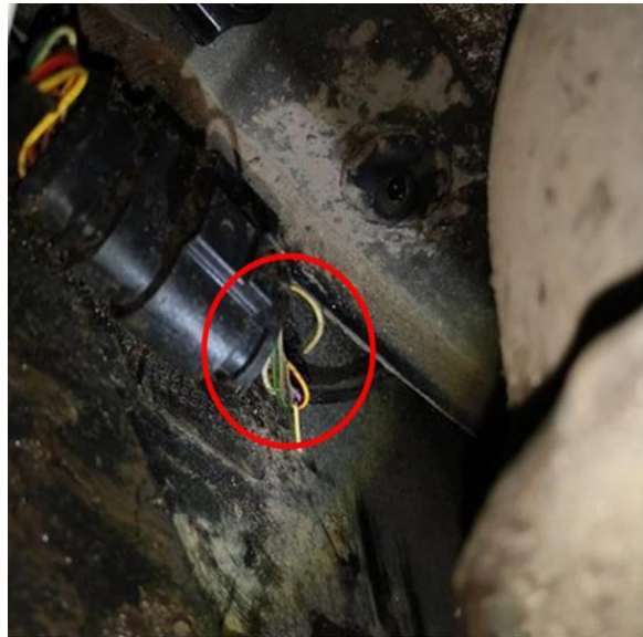
Figure 1. Location to inspect T14m for damage.
