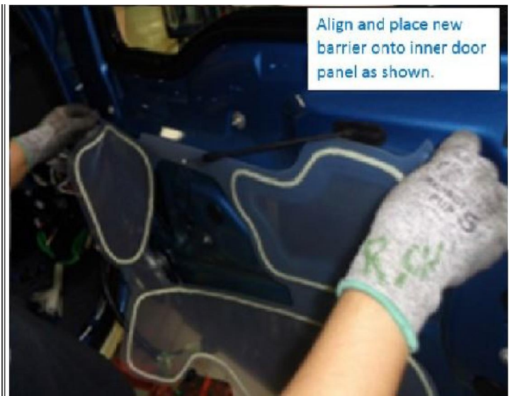
Figure 4: Plastic Vapor Barrier aligned and in place.
