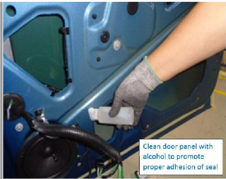
Figure 2: Cleaning the Door Panel of Old Residue
