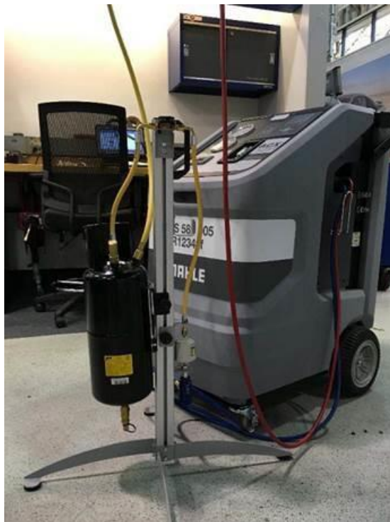
Figure 1. The VAS581005 Air Conditioning Service System with Flushing Device.
