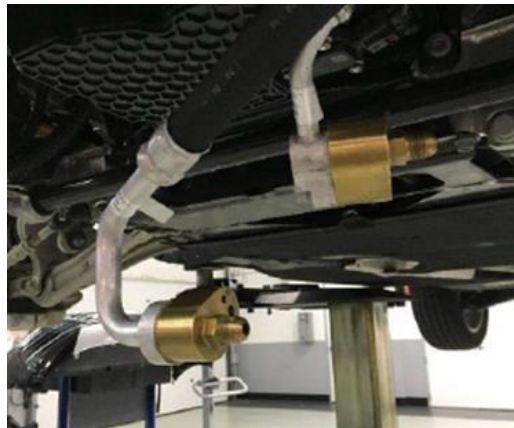
Figure 6. Installation of VAS 6338/3 and 6338/12.
