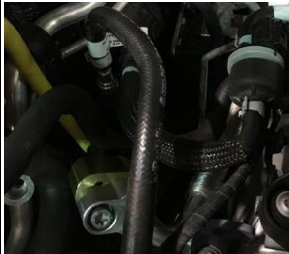
Figure 15. Attaching service station and flush hoses to rear A/C lines.
