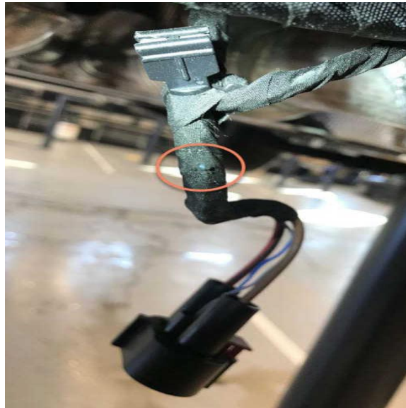
Figure 3. The damage on the original harness might be difficult to spot.
