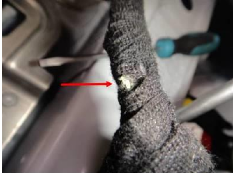
Figure 6. Shows the rub mark on the wiring harness.
