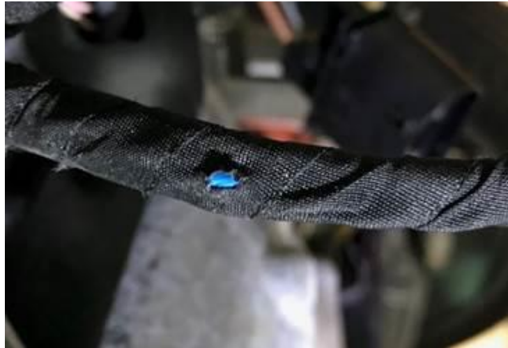
Figure 2. Example of a small rip in the protective tape.
