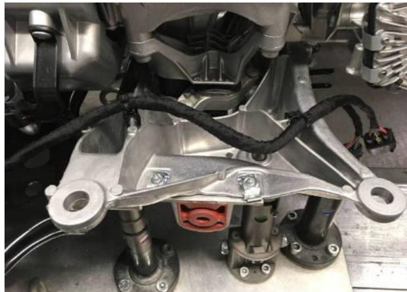
8. Routing and mounting of the transmission harness behind the crossmember.
