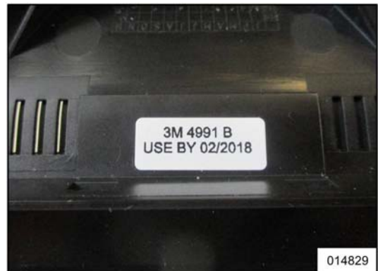
Figure 10: Mounting expiry date of support of lane-departure warning system (typical: February 2018)
