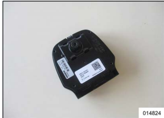
Figure 2: Wabco LDW2 lane-departure warning system camera
