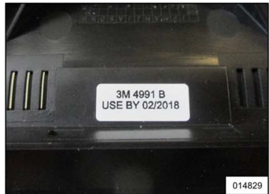
Figure 11: Mounting expiry date of support of lane-departure warning system (typical: February 2018)
