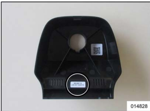
Figure 10: Location of adhesive label with expiry date on support
