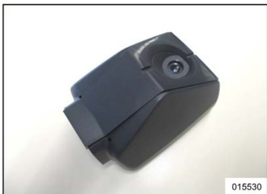
Figure 1: Iteris LDW lane-departure warning system camera
