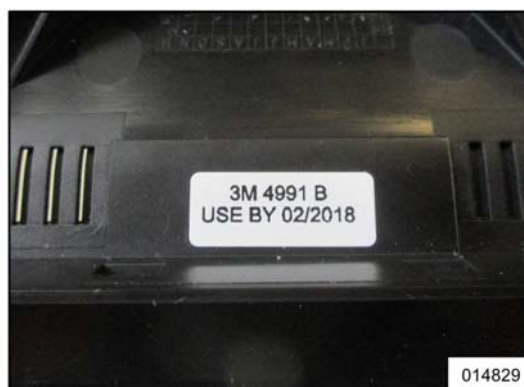
Figure 11: Mounting expiry date of support of lane-departure warning system (typical: February 2018)
