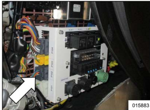
Figure 8: Connector P102 in front junction box (EKF)
