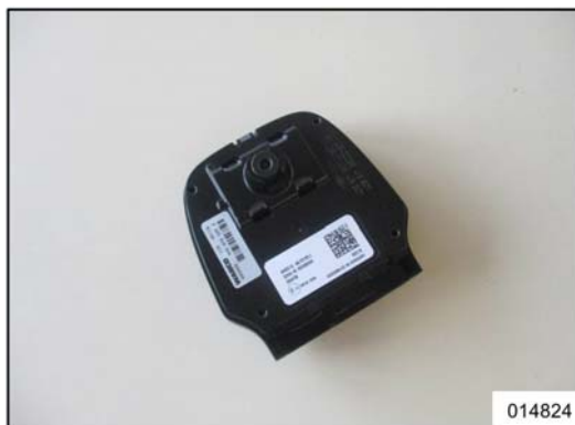
Figure 2: Wabco LDW2 lane-departure warning system camera
