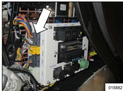
Figure 7: Connector P104 in front junction box EKF
