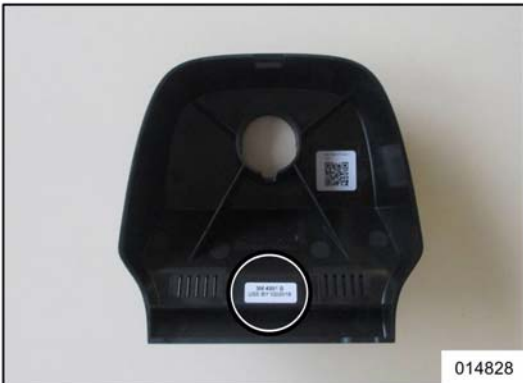
Figure 8: Location of adhesive label with expiry date on support
