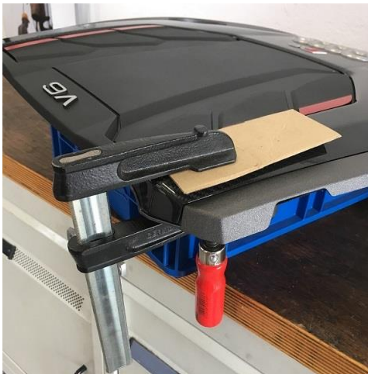
Figure 7. Put the cover in position and clamp together.
