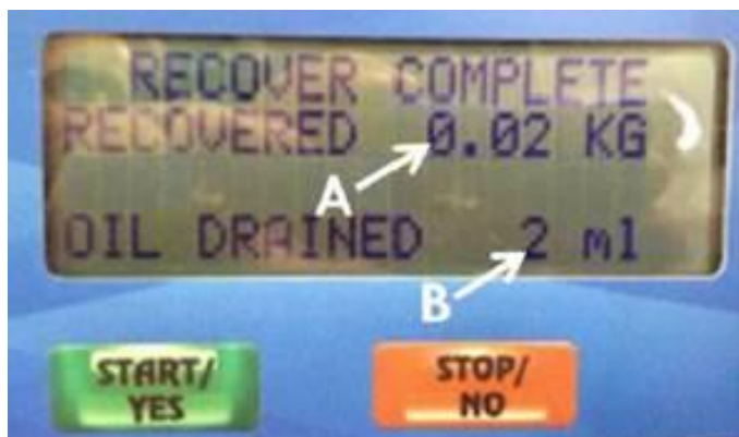
Figure 3: Amount of refrigerant recovered (A), and amount of oil drained (B).
