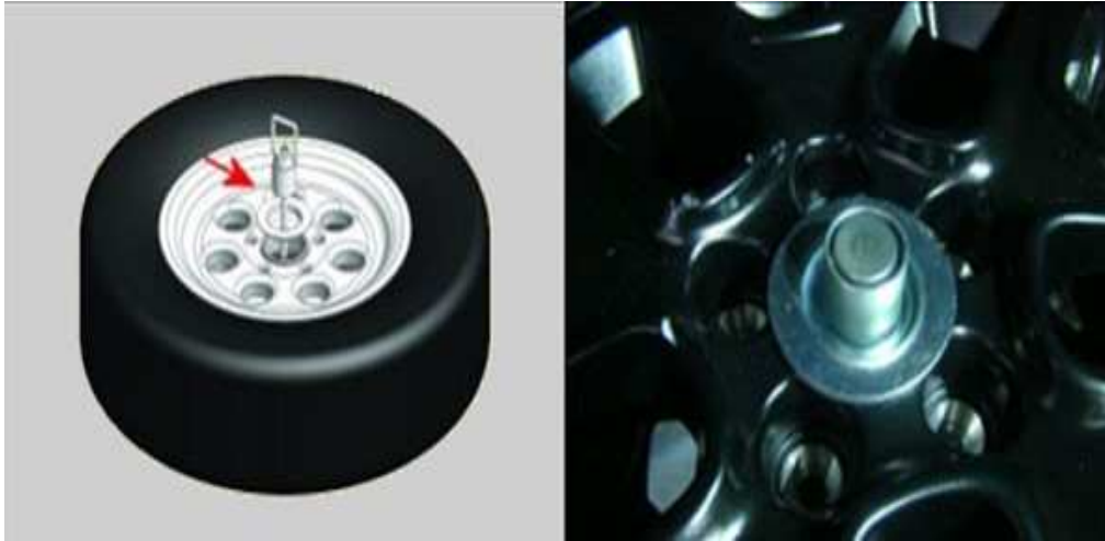
Fig. 3 Spare Wheel Anti-theft Retainer Screw
