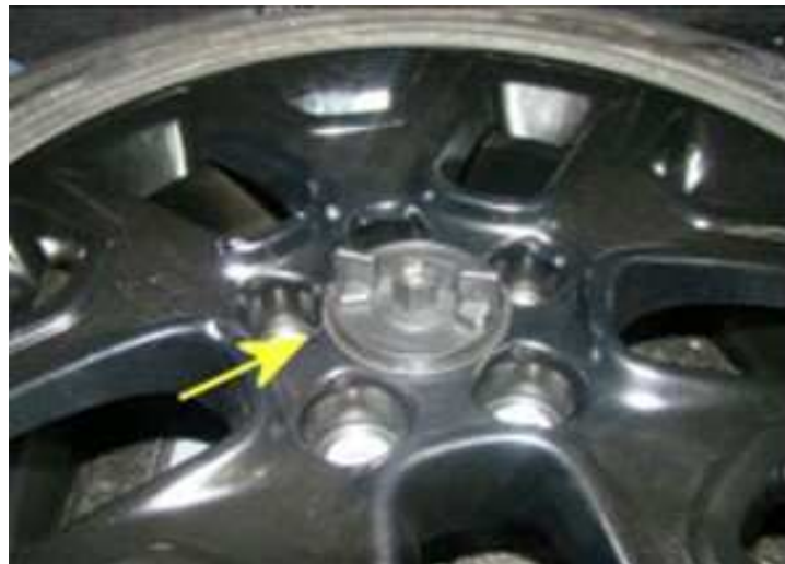
Fig. 2 Existing Spare Wheel Retainer Screw
