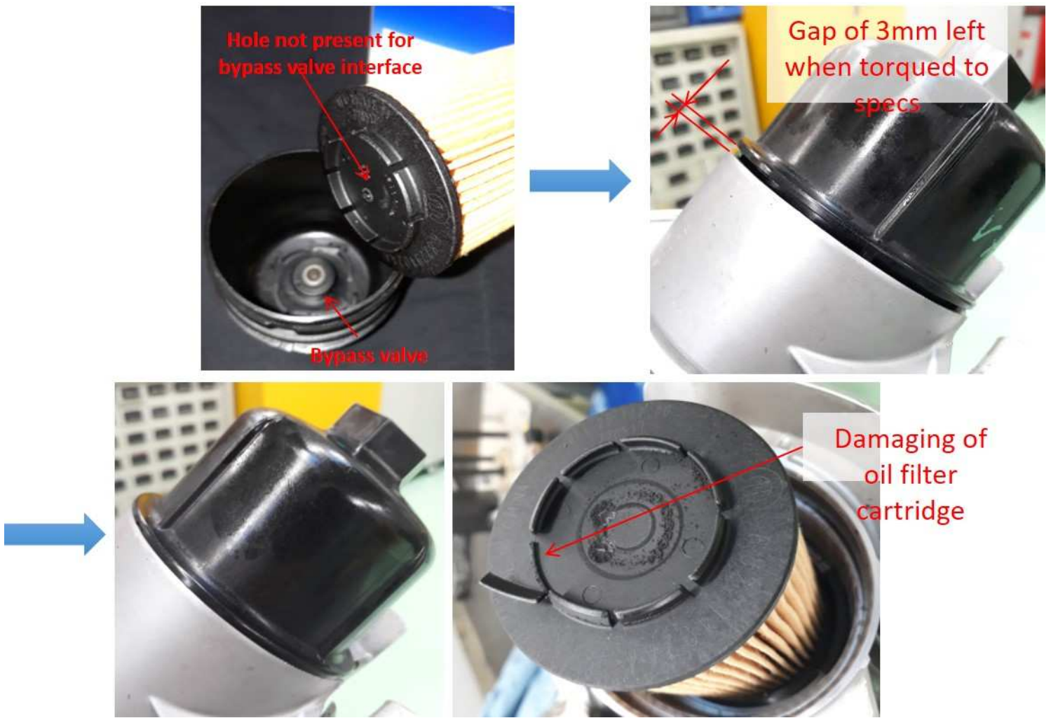
Fig. 3 Damage to the Oil Filter Cartridges
