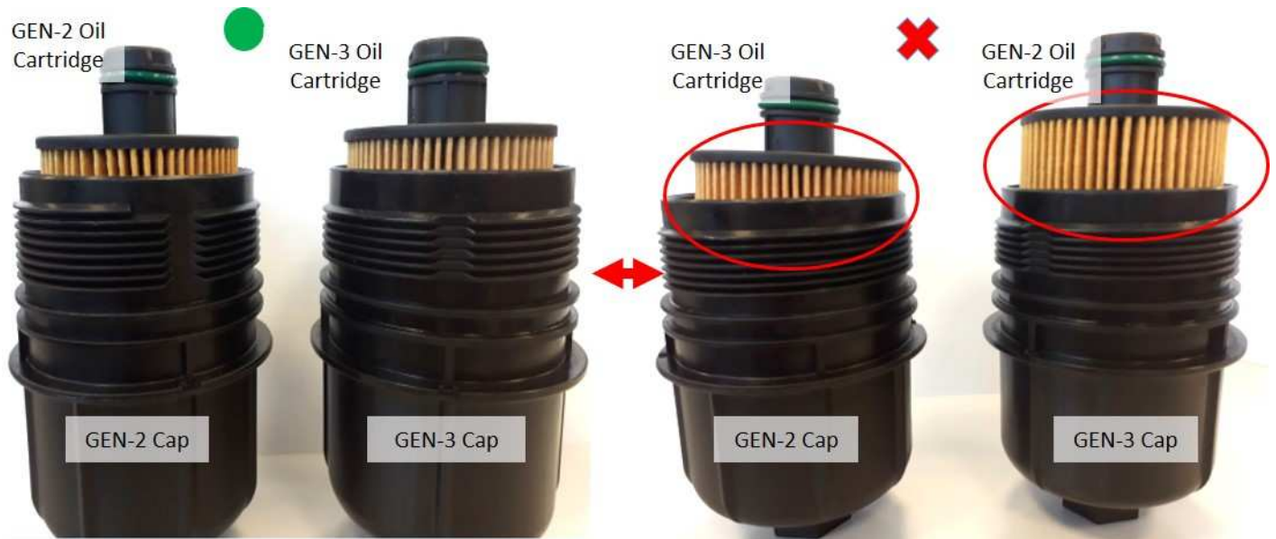
Fig. 2 Fitment of Oil Filter Cartridges in the Cap
