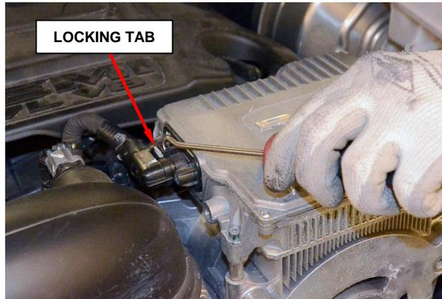
**Figure 5 – Wire Harness Connector**
