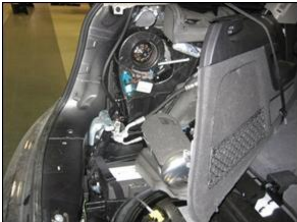
Figure 8. Location of rear air conditioning unit and expansion valve.
