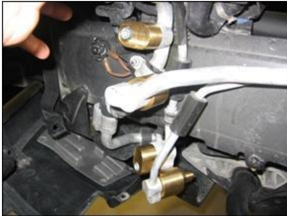
Figure 7. The location of the connections inside the left front wheelhouse on a Touareg with four zone climate control.
