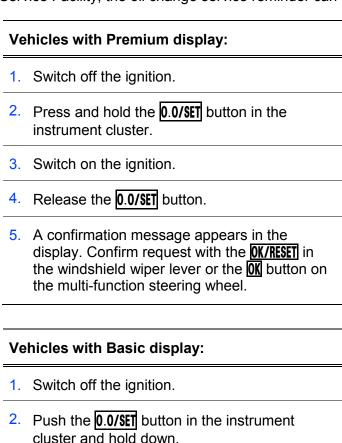
4. Release the **0.0/SET** button and push the button in the instrument cluster within about
