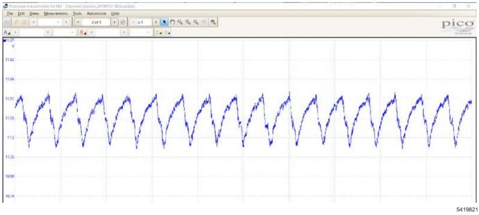
The graph above illustrates an engine that will pass a compression test and there is no reason to think that there is anything mechanically wrong with the engine.
