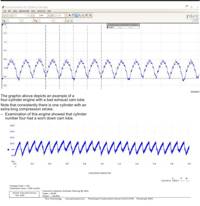
This is a four-cylinder engine with a 20 PSI loss in one cylinder
