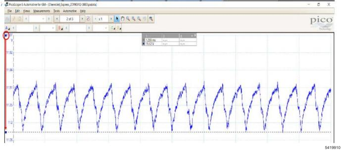
Utilizing a horizontal ruler, line up the bottom of the waveform.
