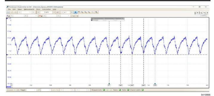
This should help to identify the top of each compression stroke in two rotations of the engine.
