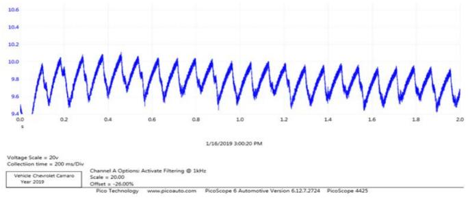
This is a four-cylinder engine with a 60 PSI loss in one cylinder.
