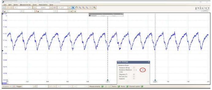
Change the rotation partition to 4, to represent the number of cylinders in the engine.
