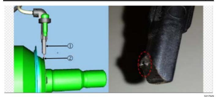
**Note:** As shown in the above illustration, the wheel speed sensor (WSS) (1) is directly in-line with the anti-click washer (2) on the outboard joint of the half shaft.
